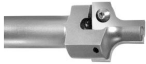
FIG. 2 Illustration of a Router Head With Insert Tooling
